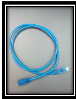
Figura 2.16 cable path cord.
