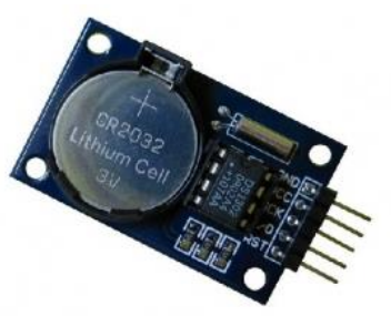
Figura 15, RTC modular, http://www.soliddepot.com/images/l/201211/13523535820.jpg .
