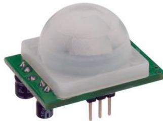
Figura 14, sensor de movimiento, http://hetpro-store.com/TUTORIALES/wp-content/uploads/2015/02/pir1.jpg
