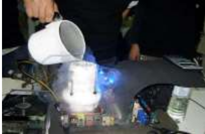
Fig. 2.14: Criogenia a motherboard
